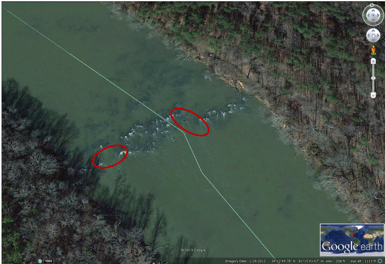
FIGURE 3-2 LEDGE 1 IDENTIFICATION AND AREAS OF NAVIGATIONAL PASSAGE (CIRCLED IN RED)
